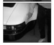
10. If you have to move the sheet metal screws to make both sides equal, DO IT! Now it's time to glue on the flare. Use a good 3M 2-part glue. Go to your auto body paint supply store and buy what they recommend. The next day, remove sheet metal screws. Grind and fill gap with Duraglass. Finish with bondo. Fill underside with seam sealer.
