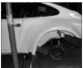
7. Attach fender flare with sheet metal screws, using level to find the same position of the top of the wheel arch.
