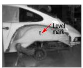
6. Grind off paint in preparation to glue on fender flare. You can use a flange air tool to put a 90° jog in the quarter panel. The advantage of using this tool is that you don't have to use as much filler.
