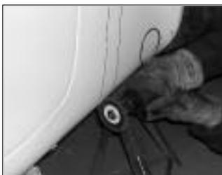
4. Use a cut-off tool to cut old quarter panel off of the car. Use cut-off wheel, air chisel, or plasma cutter.
